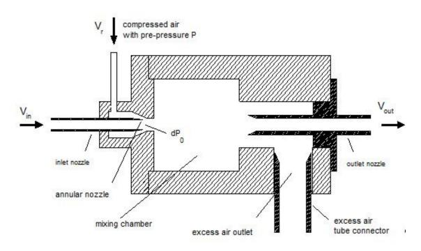
Particle-free air with the volume flow  $V_R$  circulates through an annular passage around the suction nozzle. Thus, according to Bernoulli, a volume flow  $V_{An}$  is generated at the suction nozzle.
