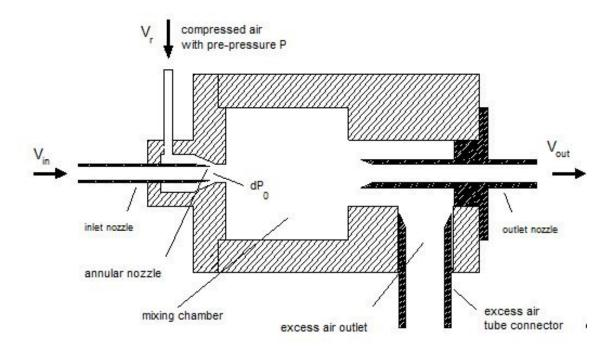
Particle-free air with the volume flow  $V_R$  circulates through an annular passage around the suction nozzle. Thus, according to Bernoulli, a volume flow  $V_{An}$  is generated at the suction nozzle.
