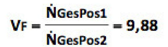
Provided the first measurement is not affected by a coincidence error and the dilution system under test is working (not soiled), a dilution factor of almost 10 is determined. If this should not be the case, there was possibly coincidence in measurement 1. In this case the aerosol concentration has to be decreased or a further dilution step used. Another possibility would be that the dilution step to be tested is soiled. In this case the device has to be cleaned and the test repeated.
